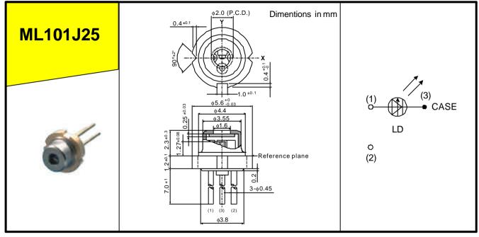
There is no model with a monitor photo diode in ML1XX25 series.
